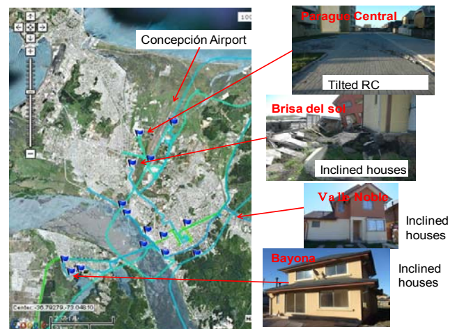
Fig. 3 Sites of liquefaction damage in Concepción
