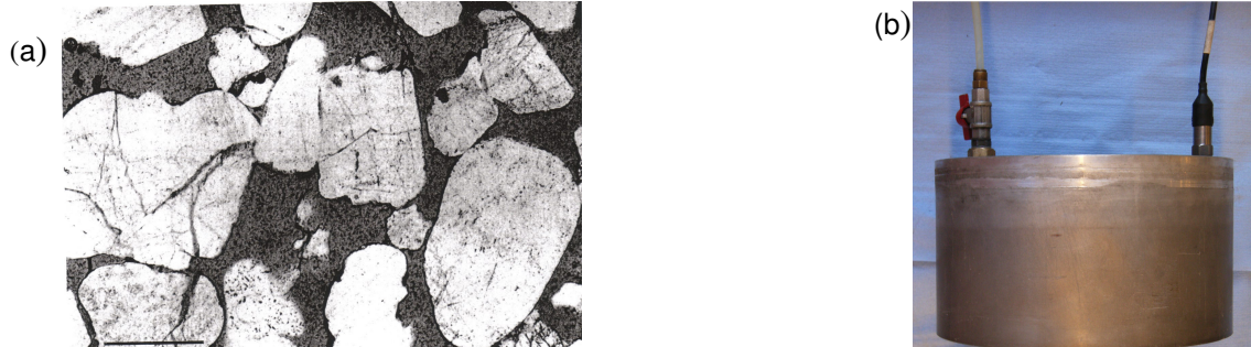
Figure 5: (a) Photomicrograph by Richards and Barton (1999). The scale bar is approximately 0.3 mm in length, and (b) caisson model showing fluid valve and pore pressure transducer
