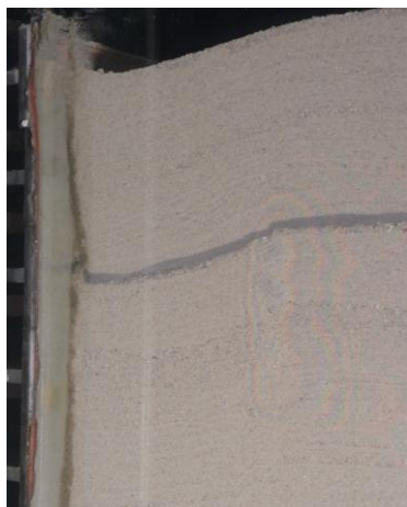
Figure 3: Distortion detail of the geogrid and soil settlement
