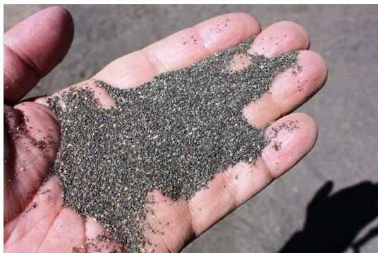
Figure 7: Sand found at crack bottom with grain size distribution inside highly liquefiable range
